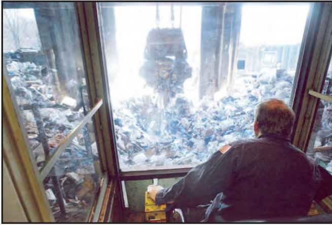
Crane operator Tom Johnson hoists household garbage to be burned and converted to energy in the Pittsfield Resource Recovery Facility on Thursday.
